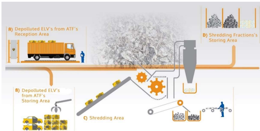
Figure 8. Shredding facility typical layout (Source: SIGRAUTO)
