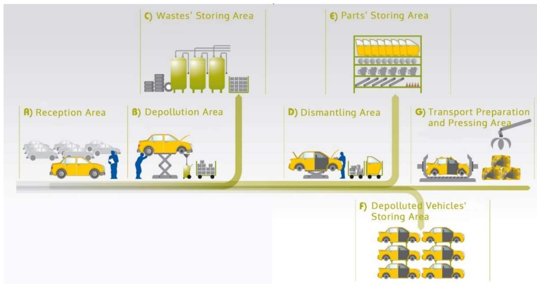
Figure 7. Illustration for a typical layout of an ATF (Source: SIGRAUTO)
